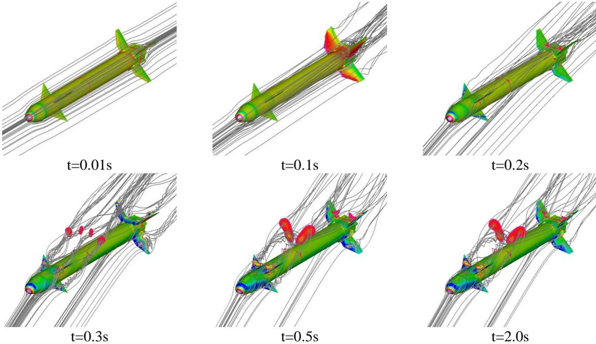
Figure 15. The spatial streamlines for Case6 at different times
