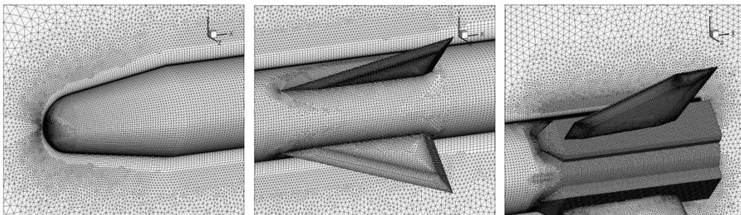
Figure 3. The initial grids over the missile model
