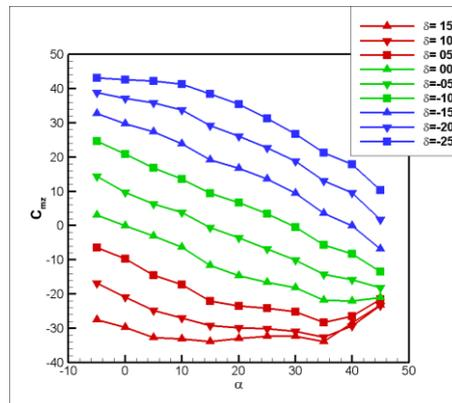
Figure 7. The static moment coefficients with different angles of attack of the missile and deflection angles of the rudders
