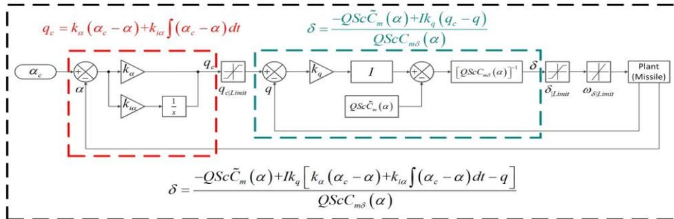
Figure 6. Sketch of the flight control system
