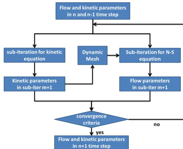
Figure 5. Sub-iteration procedure of the strong coupled solver.
