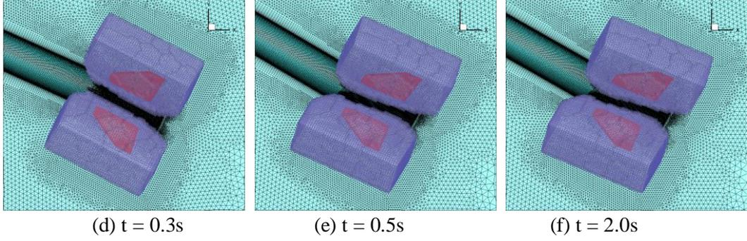
Figure 4. The dynamic overlapping grids over the deflecting rudders.
