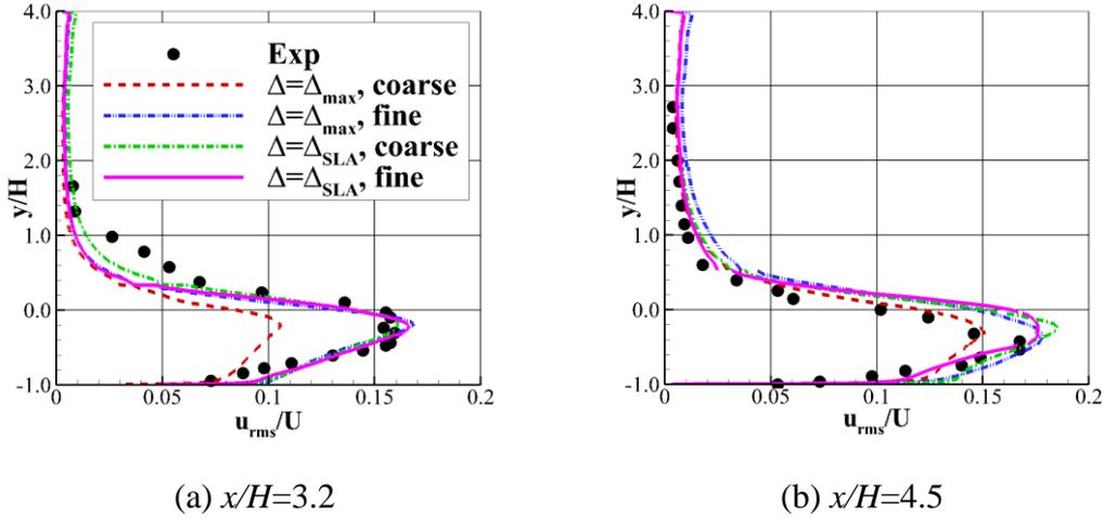
Figure 5 Streamwise velocity fluctuations at two streamwise locations from standard IDDES and IDDES with  $\Delta = \Delta_{SLA}$
