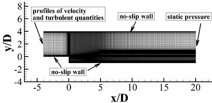
Figure 3 Computational domain and boundary conditions
