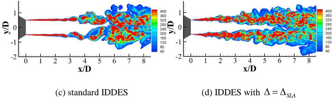
Figure 2 Instantaneous fields of eddy viscosity  $\mu_t/\mu$  (upper) and vorticity magnitude (lower) calculated from standard IDDES and IDDES with  $\Delta = \Delta_{SLA}$  on the fine grid
