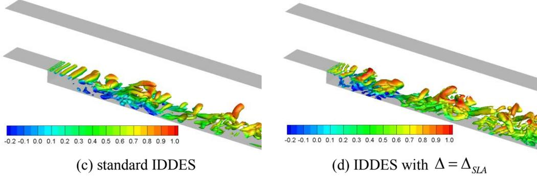
Figure 4 Instantaneous eddy viscosity (upper) and iso-surface  $Q(H/U)^2 = 0.1$  (lower) on the coarse grid
