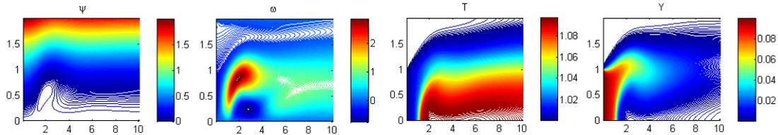
Vortex breakdown develops sooner with the presence of combustion and this matches known results [2]. It is observed that the mixing due to vortex breakdown greatly affects the temperature such that a local temperature maximum is coincident with a vortex bubble center. Understanding how instabilities are effected by geometry and reactant consumption are the main goals of this study and several examples will be presented in the final paper.
