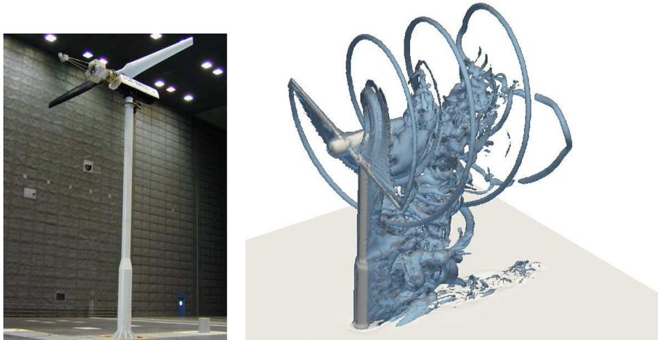
Figure 1: NREL turbine. Left, real turbine (<http://www.nrel.gov/data/pix/Jpegs/17305.jpg>). Right: numerical solution of the flow (norm of vorticity).
