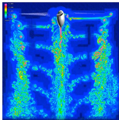
**Figure 3** OVERFLOW AMR hover simulation,  $M_{tip}=0.625$ ,  $Re=2.1$  million.
