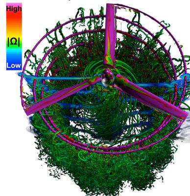
**Figure 4** OVERFLOW AMR hover simulation,  $M_{tip}=0.625$ ,  $Re=2.1$  million.
