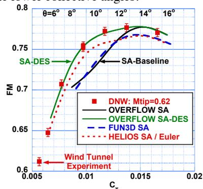
**Figure 2** OVERFLOW simulation of the V22 rotor in hover,  $M_{tip}=0.625$ ,  $Re=2.1$  million.
