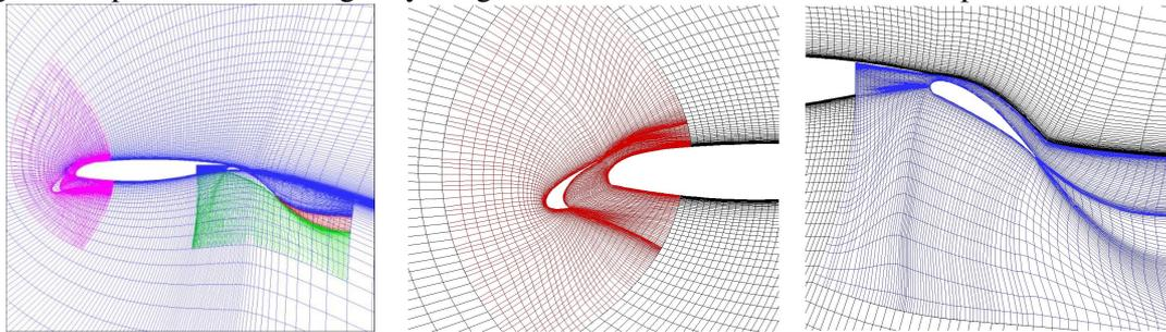
Figure 2: Geometry definition of the high-lift airfoil
