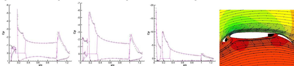
Figure 3: Validation of the NSAWET code and Window-Embedment grid by MD 3-element airfoil
