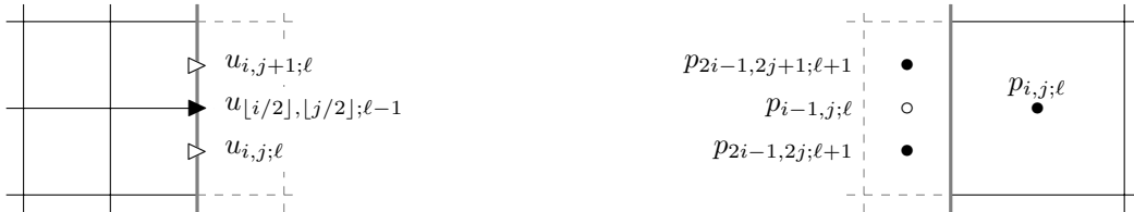
Figure 10: Left : missing variables ( \triangleright ) for the divergence operator, together with the variable used for constant extrapolation ( \blacktriangleright ). Right : Missing variable ( \circ ) for the gradient operator, together with the variables used for linear interpolation ( \bullet )
