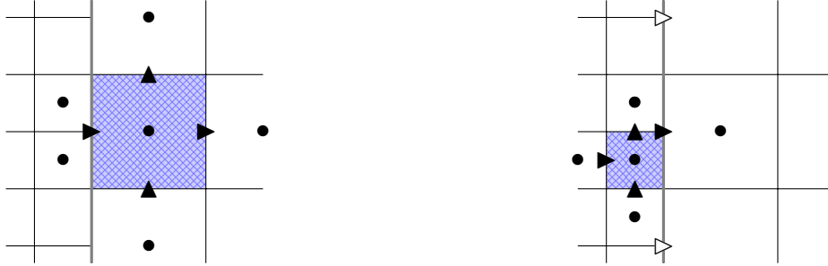
Figure 12: Visualization of the pressure Poisson stencil for the discretization given by (37). The velocity variables \blacktriangleright and \blacktriangle are used in M\mathbf{u}_h^{n+1} . The actual Poisson stencil for MGP_h^{n+1} consists of the pressure variables \bullet . Note that the variables \triangleright are only used on the right hand side in the term M^+\mathbf{u}_h^* .
