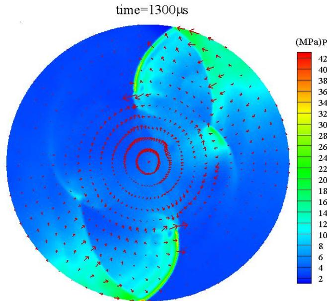
Fig.9 Pressure contour on an axial slice at  $z=0.2\text{cm}$  at 1300 $\mu\text{s}$
