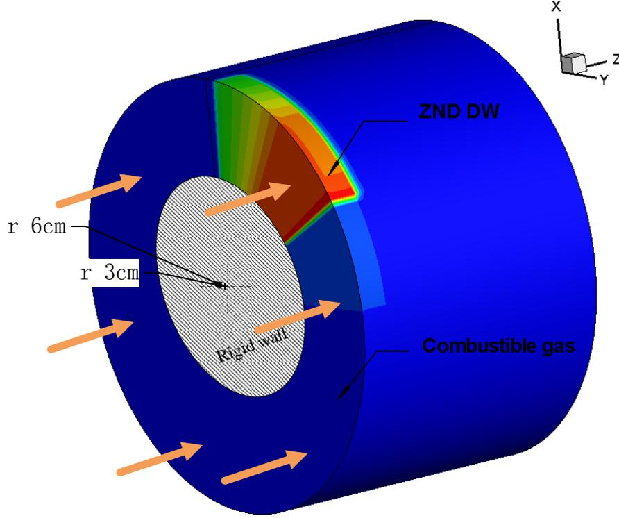
Fig.1 Initial conditions in the hollow combustion chamber
