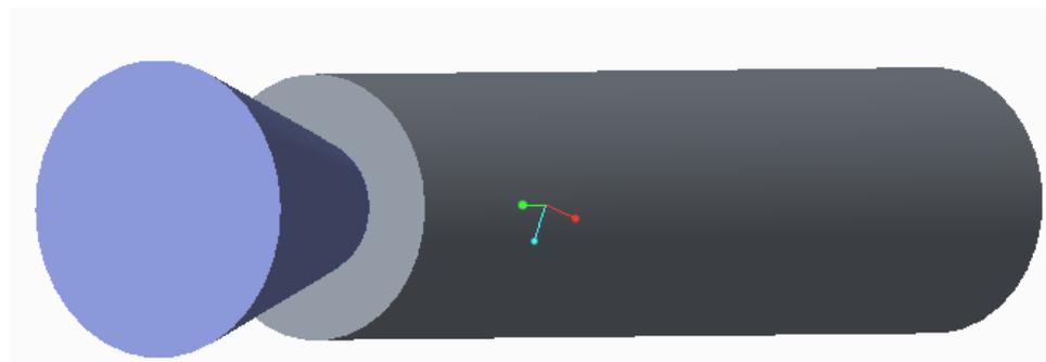
Figure 1. Axisymmetric dump combustor configuration for the baseline configuration
