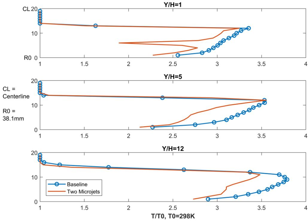
Figure 5. Mean Static Temperature along the radial axis at different axial sections of the combustor at  $t=0.3\text{ s}$ ,  $T_0=298\text{K}$
