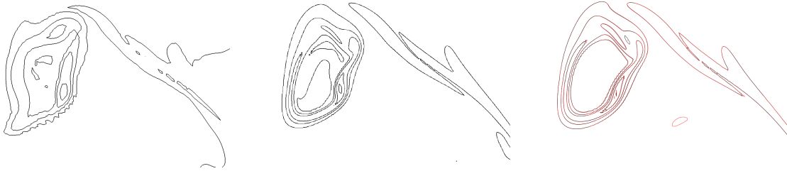
Figure 4: Contours of vorticity norm at T = 8 in the YZ plane at x = 0 in a 2\pi -long cubic domain obtained with the present eddy viscosity model with a 256^3 - 64^3 resolution (left) and a 512^3 - 128^3 resolution (center). They are compared to the DNS results obtained by [10] with a 512^3 resolution (right).
