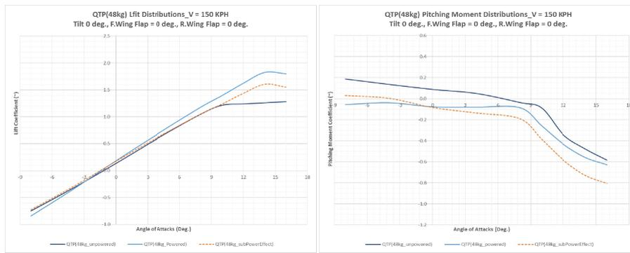
**Figure 8 : Numerical results of powered model, left: lift coefficient, right: pitching moment coefficient**
