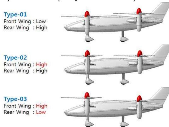
**Figure 3:** Vertical position variation of front and rear wing. Type-1: low front wing & high rear wing, Type-2 : high front wing & high rear wing, Type-3 : high front wing & low rear wing
