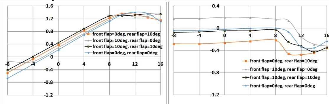
Figure 6: Lift(left) and pitching moment(right) coefficient distribution with deflected flaps
