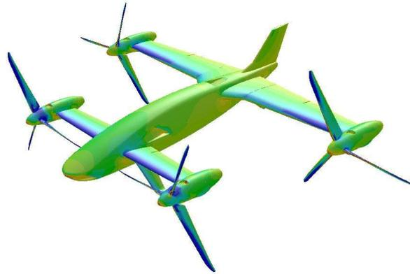
**Figure 7 : Pressure contour of powered model, blue : low pressure**
