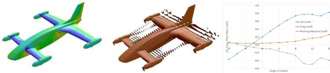
**Figure 2:** Numerical results of unpowered model, left: surface pressure contour, center: low speed contour around vehicle, angle of attack=8°, right: aerodynamic characteristics
