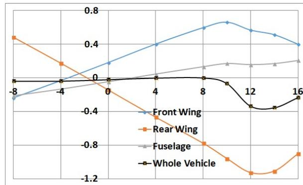
Figure 5: Pitching moment distribution for the decreased area and increased incidence angle of rear wing
