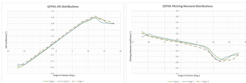
**Figure 4:** Lift and pitching moment distribution versus angle of attack for vertically varied front and rear wing positions
