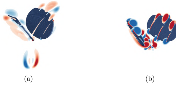
Figure 12: Normalized spanwise vorticity at the end of peel phase at location 0.2R, 0.5R and 0.8R from the wing root for (a) \xi = 0\% and (b) 100%
