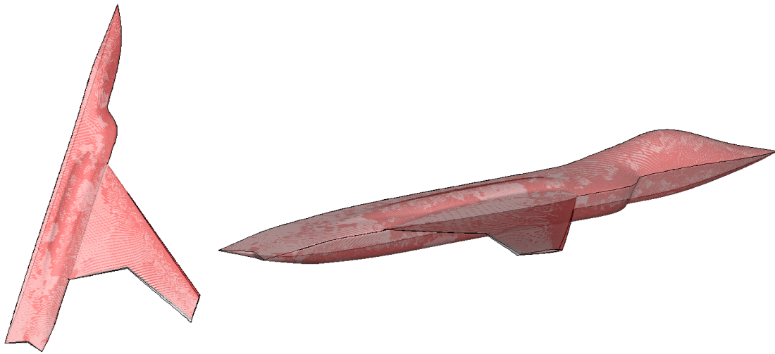
Figure 12: Initial (white) and optimal (red) aeroelastically deformed shapes for the lift- and moment-constrained drag minimization.
