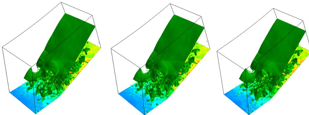
Figure 6: The 3-D shape of the distorted shock wave by the iso-surface of  $|\nabla p|$
