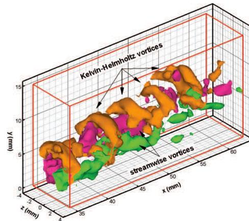
Fig. 4 K-H rings behind MVG by Experiment (Sun et al 2011)
