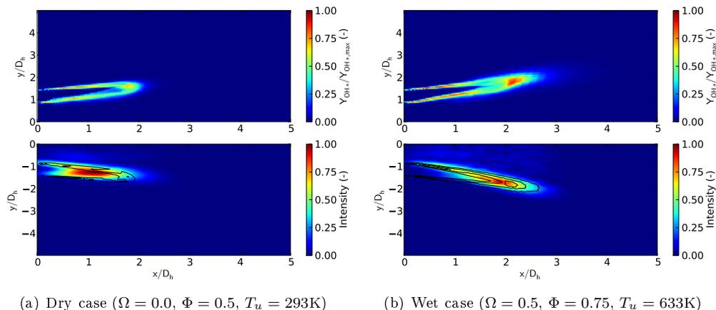
Figure 1: Comparison of the LES (top) with experimental OH\* chemiluminescence measurements (bottom).
