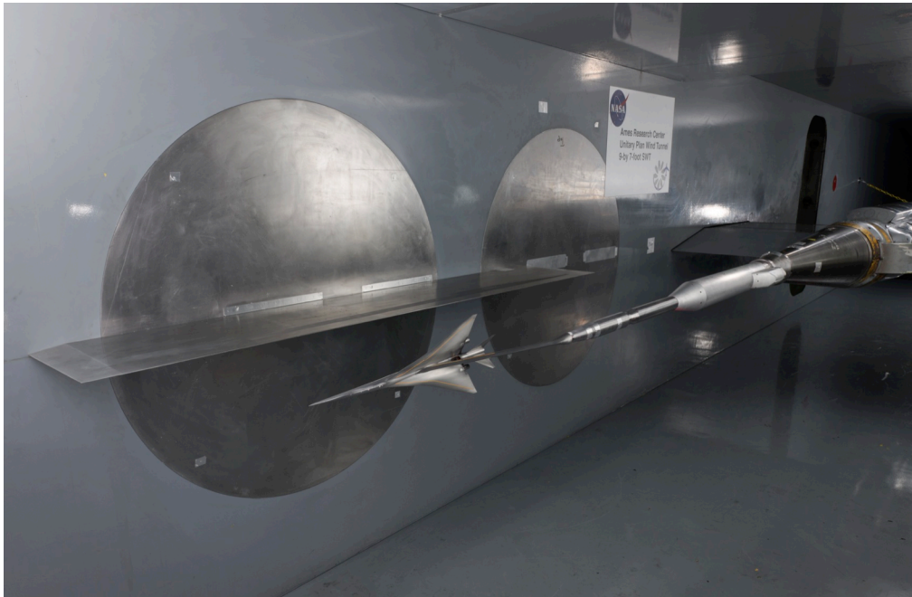
Figure 6: Photograph of the RF 1.0 rail attached to the forward window blank in the 9x7 Wind Tunnel.
