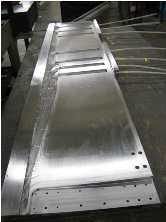
Figure 5: Photograph of the RF 1.0 rail showing the routing of 420 metal pressure tubes channeled through machined grooves on one surface of the rail.
