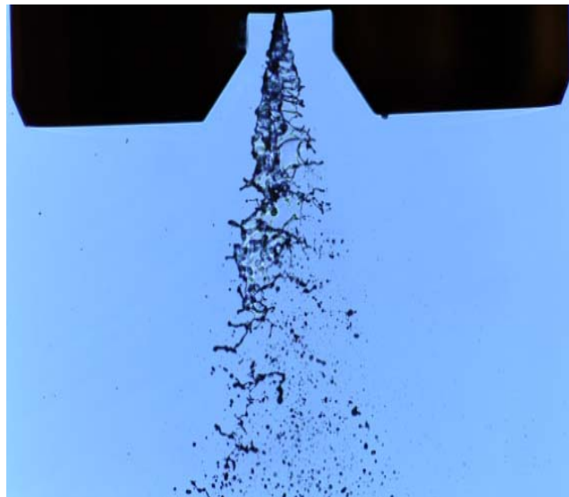
Figure 3: Liquid jet experimental view from a compound nozzle (Triballier et al [19])
