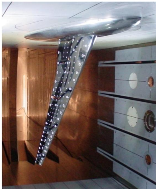
Figure 6: HIRENASD wing mounted in the European Transonic Wind Tunnel.
