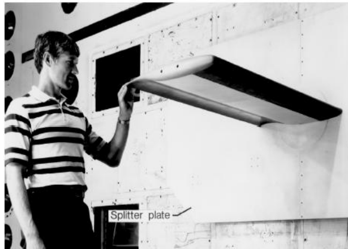
Figure 2: Rectangular Supercritical Wing mounted in the NASA Langley Transonic Dynamics Tunnel.
